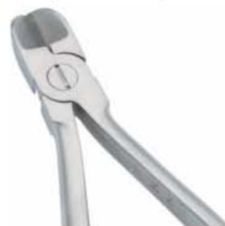
L5-008 Hard wire cutter, easily cuts any size arch wire or pin. The inserted tips ensure precision cutting and perfect tip alignment. Minimum Cutting Capacity: .012"(.30mm) Maximum Cutting Capacity: arch wires up to .021"x.025"(.55mmx.64mm)
